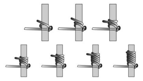
d. Keeping tension on the rope, tie a series of rolling hitches (#1734 suggested) until all of the tail is used.
