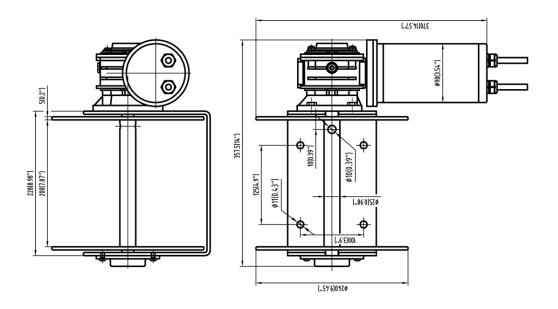
Dimensional Drawings for Savwinch 1000CS/SS/SSS
