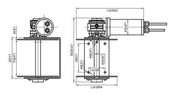
Dimensional Drawings for Savwinch 880CS/SS
