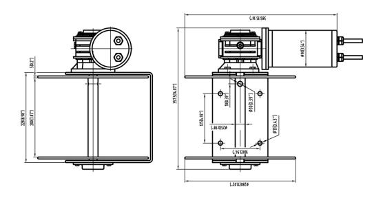
Dimensional Drawings for Savwinch 1500CS/SS/SSS
